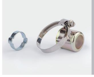
To fix hoses to fittings, different assembly methods can be used ranging from robust clamps to light clips to ferrules. The assembly method depends on the application, media, pressure or hose material. Criteria are: safety level of fixation, removability, easiness and devices needed for assembly as well as cleanliness and protection against injury.
