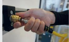
To disconnect, pull back the sleeve of the coupling (comes with automatic locking mechanism in shut-off couplings and plugs)
